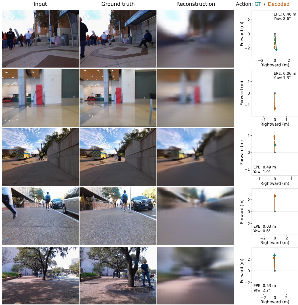
Figure 17: Qualitative results of our LAM on SCAND. Each row shows the input image, ground-truth target image, reconstruction, and ground-truth versus decoded actions. Endpoint error (EPE, m) and yaw error ( ^{\circ} ) are reported for each example.
