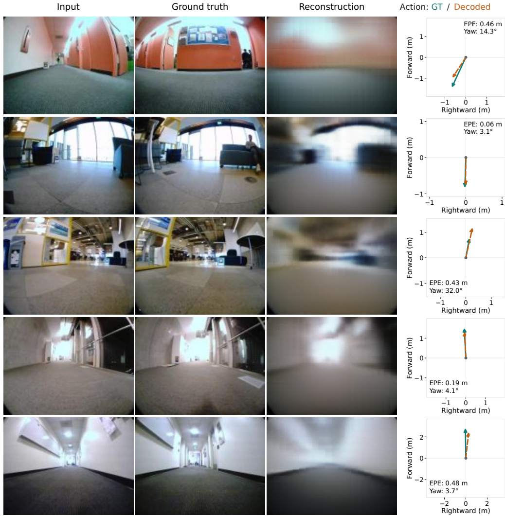
Figure 15: Qualitative results of our LAM on HuRoN. Each row shows the input image, ground-truth target image, reconstruction, and ground-truth versus decoded actions. Endpoint error (EPE, m) and yaw error ( ^{\circ} ) are reported for each example.
